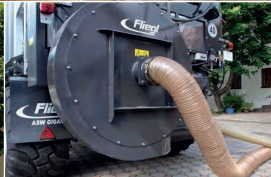
New High Performance Blower Ø 1200 mm with:
